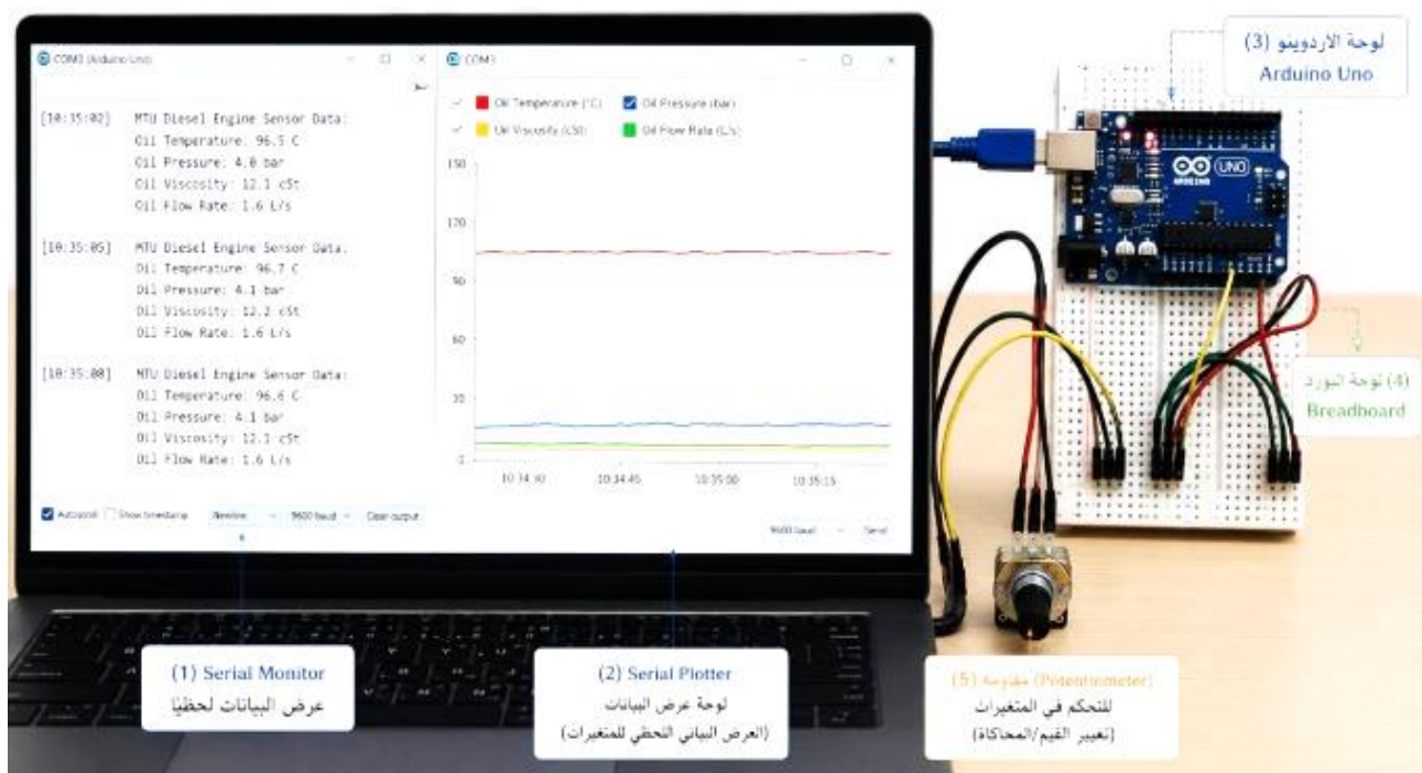
Figure (2): Monitoring-system interface and data display (Serial Monitor) and model components [8,9].
