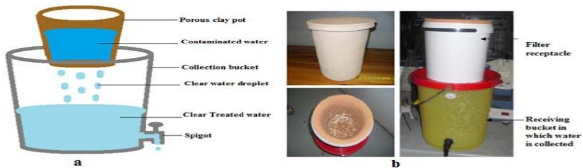
Figure 7 Porous pot filter design and treated-water collection. Source: (Mwabi et al., 2012)
