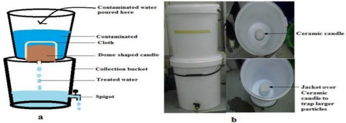
Figure 6 Ceramic candle filter design and housing. Source: (Mwabi et al., 2012)
